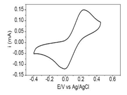
Voltammograms of printed line-electrodes in a 10 mM K4[Fe(CN)6] solution.
