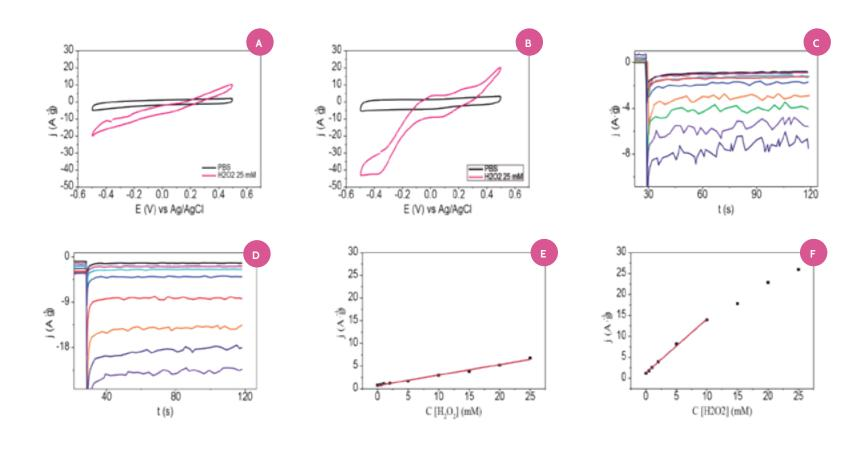
A-B) Cyclic voltammetry for T1 and T2 samples, respectively. C-D) Chronoamperometry at -0.3 V for H<sub>2</sub>O<sub>2</sub> concentrations between 0.5 and 25 mM, for T1 and T2, respectively. E-F) Calibration curves obtained for T1 and T2, respectively.
